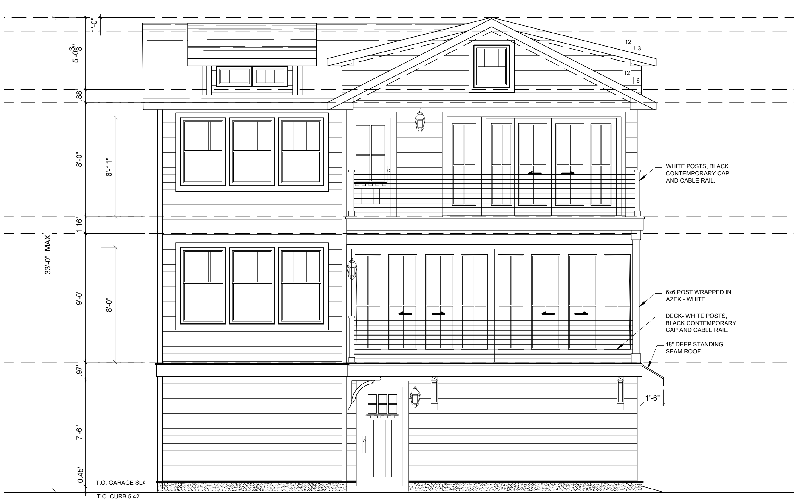
PROPOSED FRONT ELEVATION (FIRST AVE.) SCALE: 1/4"=1'-0"
